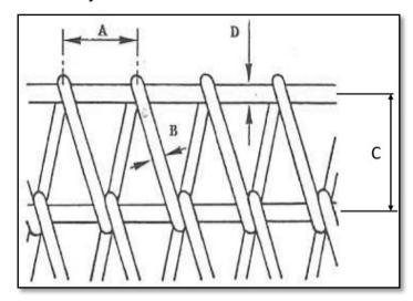
**NOTE:** When measuring pitches A & C, it is best practice to measure over 10 pitches and then divide by 10 to obtain the average pitch.
